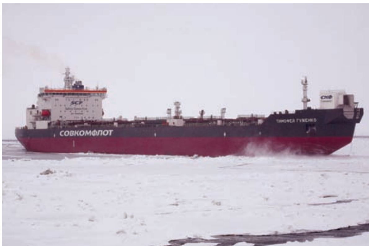
Timofey Guzhenko is the last of a trio of Arctic shuttle tankers and has been fitted with a unique ice load monitoring system.
